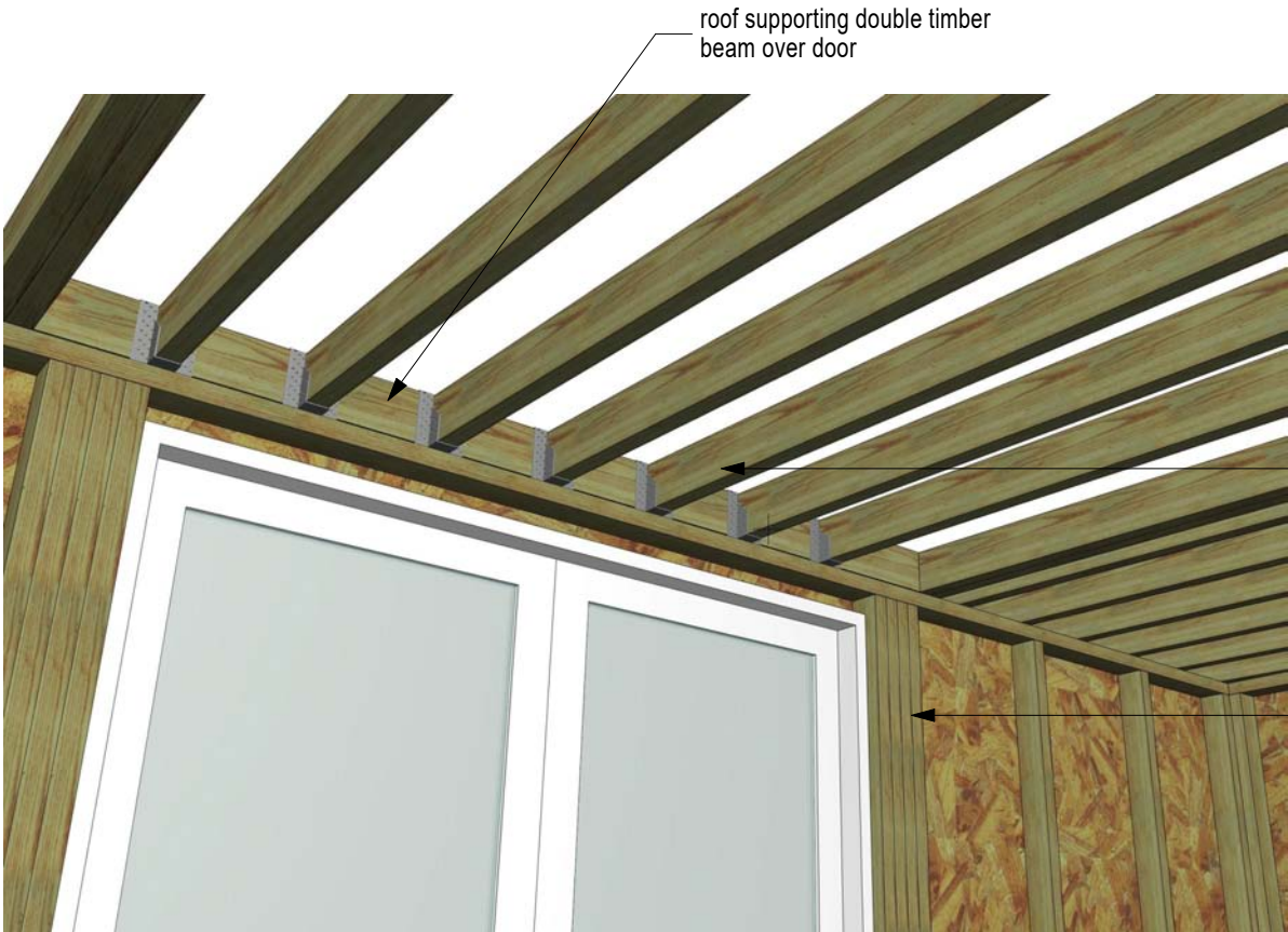
ceiling joist supporting detail
